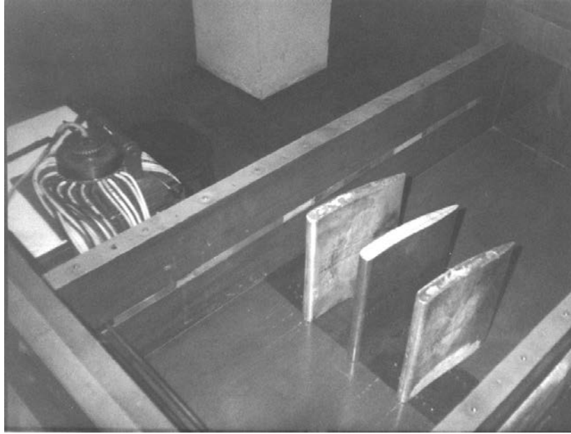
Fig.1.2 Cascade of S profiles for t/l of 0.62 and attack angle \alpha=5^\circ
