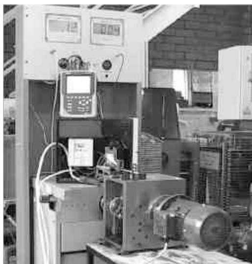
Fig. 6.2 The gearless, clutchless non-synchronous transmission
