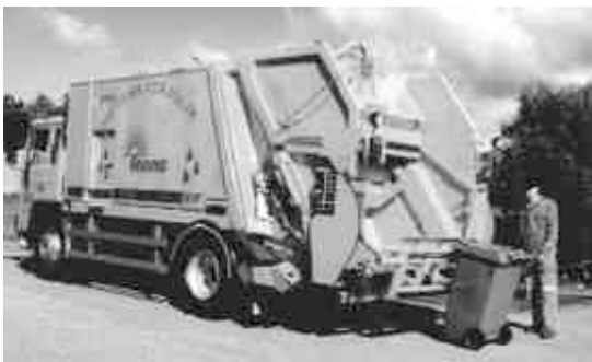
Fig 13. Municipal vehicles in which all cylinders are powered and controlled by water hydraulics systems
