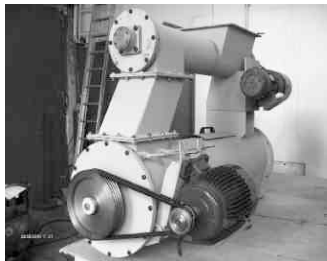
Picture. 1. Fuelling, homogenisation and dosage mechanism
