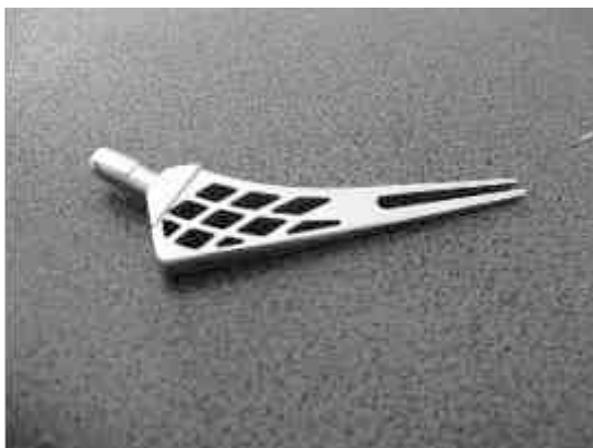
Figure 15. Examples of parts built in EOS superalloy CoCrMP1 on INCDMTM
