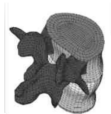
Figure 7. CAD model on human vertebrae used for FEM analysis
