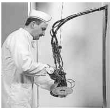
Fig.10. Energy –saving and ergonomic saw driven by a water hydraulic system
