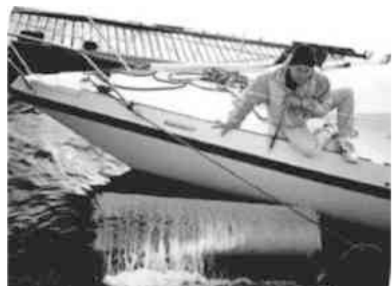
Fig 14. Yacht washing installation, without the need of a dry dock.
