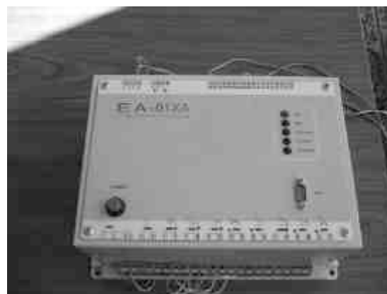
Figure 1. Modular portable data acquisition system
