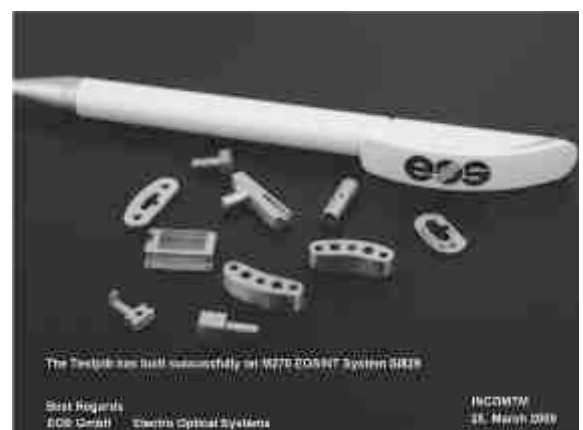
Figure 17. Examples of parts built in EOS superalloy CoCr MP1 on INCDMTM for orthopedy, neurosurgery and maxilofacial implants
