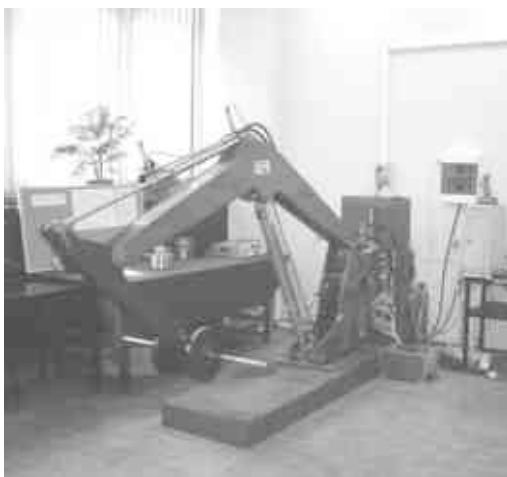
Fig 15. Experimental setup for testing a water hydraulic installation having the structure of a typical construction manipulator
