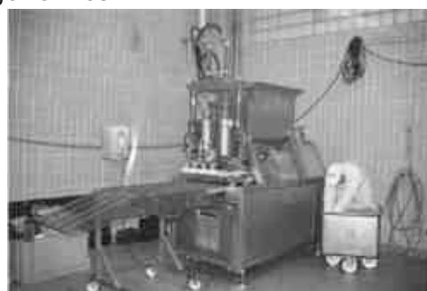
Fig 11. Hamburger forming machine driven by Nessie water hydraulic components and diagram showing the principle of water hydraulic system
