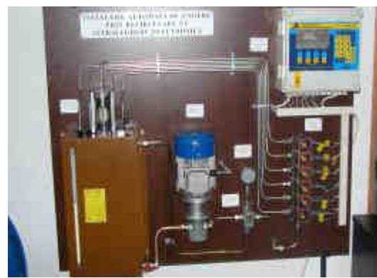
Figure 19: The recirculation lubrication system with electronic monitoring
