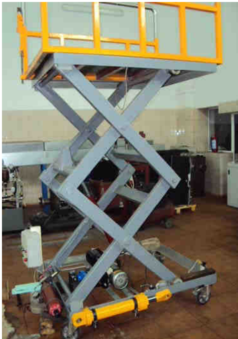
Fig. 3 Lifting platform with potential energy recovery system
