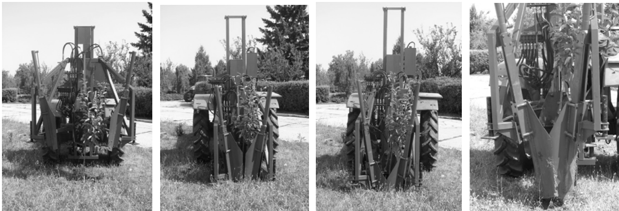
Figure 2. Aspects of the phases of working process during extraction of the root ball plants
