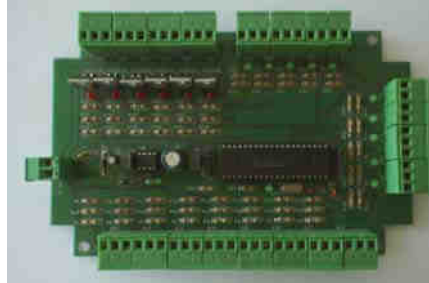
Figure 3 – Digital control module: assembled PCB TOP view.
