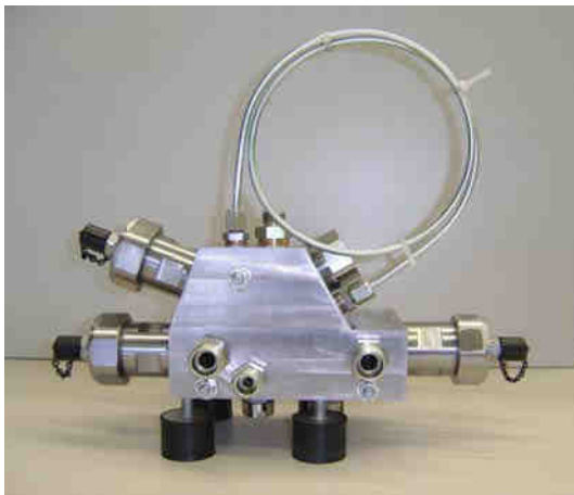
Figure 5: HBC prototype and its steady state efficiency results; (system data: inductance pipe: length: 1.2 m, diameter 3 mm, oil: Shell Tellus 15 cSt @ 40°C; switching valves: LCM FSVi ( Q_N=10 l/min @ 5 bar); switching frequency: 100 Hz; accumulators: piston accumulators, developed by the authors; find all data in [22] and [24]).
