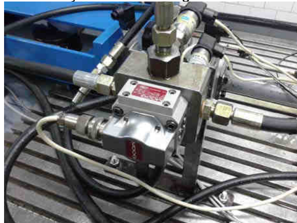
Fig. 3 Servo valve mounted on stand for testing
