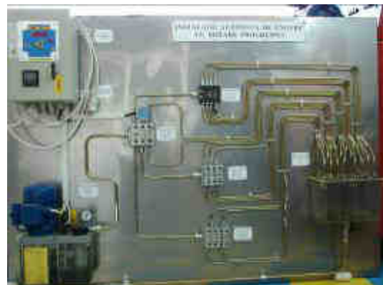
Figure 17: The progressive dosing lubrication systems
