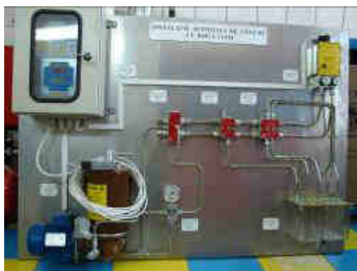
Figure 18: The lubrication systems with two lines
