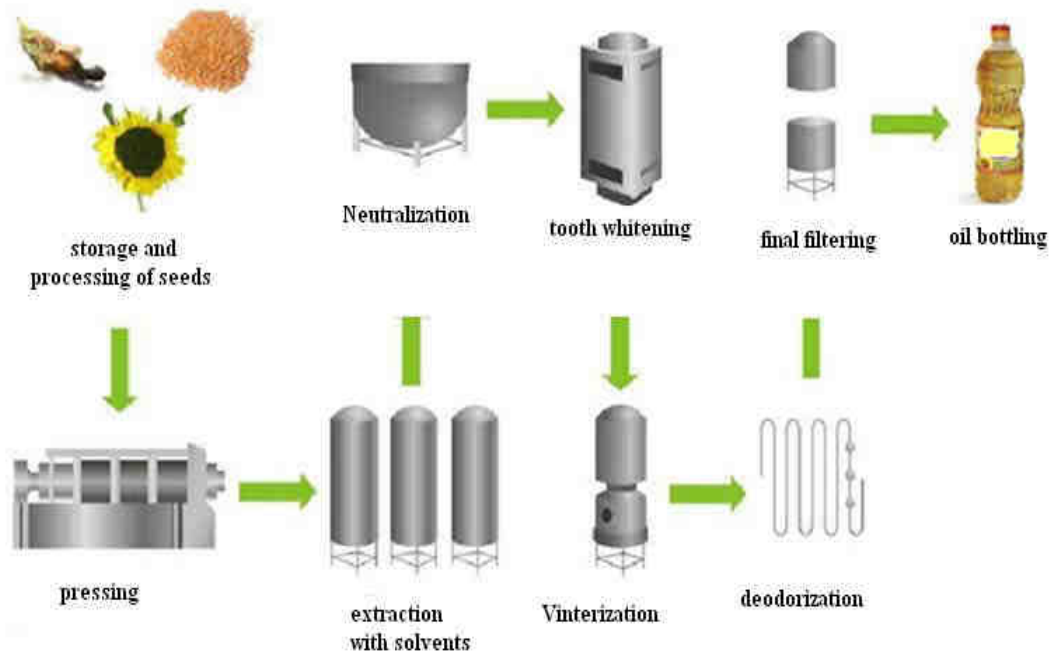
Fig.1 Technological Process Flow for Vegetable Oil
