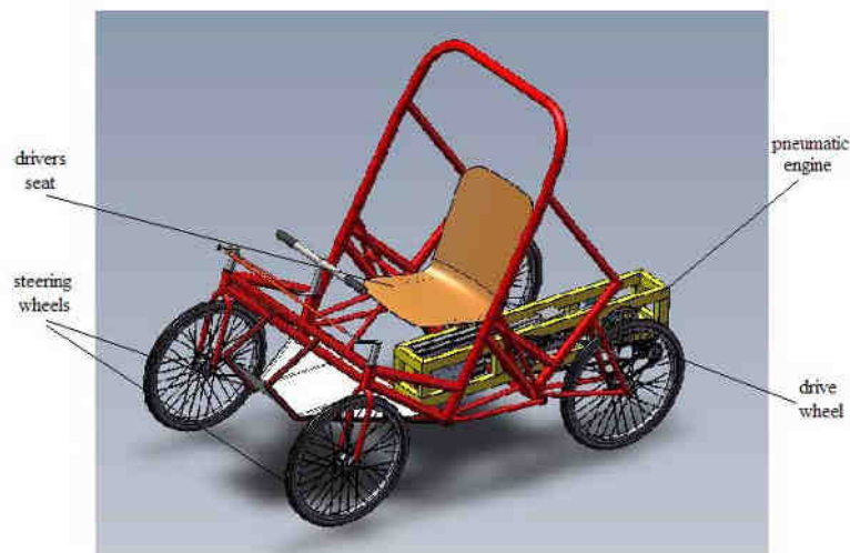
Figure 7. The construction of the pneumo-vehicle
