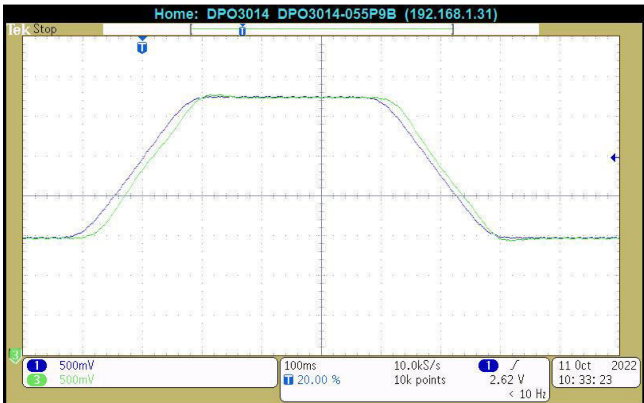
Fig. 10. Reference and actual value of position, 70 mm step, 2-DOF PI regulator and S-curve generator on set-point path K_P=4 , T_I=100 ms, K_F=10 , v_{max}=0.4 m/s, a_{max}=20 m/s 2 , j_{max}=175 m/s 3
