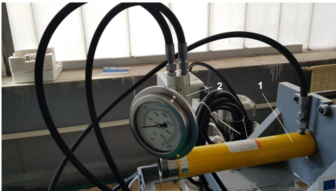
Fig. 5. High-pressure test cylinder (1), powered by the minibooster (2) equipping the low-pressure pumping unit
