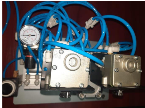
Fig. 3. The pneumatic drive system of the wire microdeformation equipment
