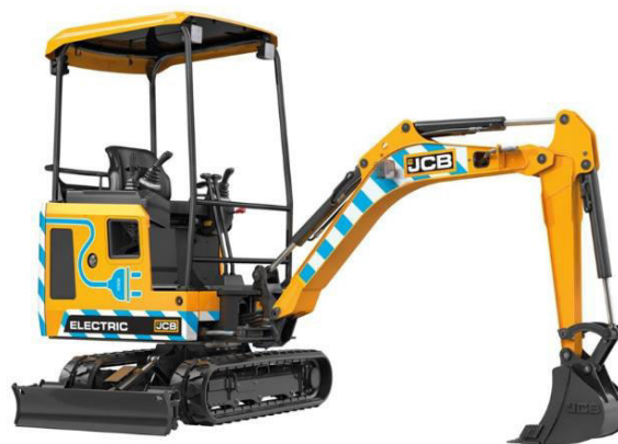
Fig. 3. The 19C-IE electric compact excavator
