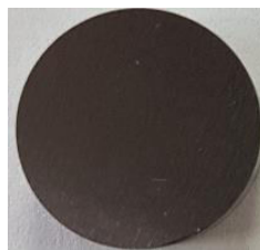
1 \mu\text{m} \text{CrN} deposited on CoCr by DC sputtering
