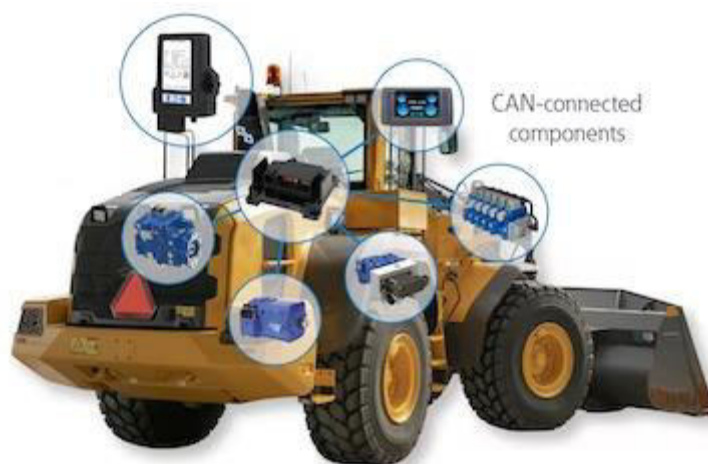
Fig. 4. Intelligent hydraulic drive system [1]
