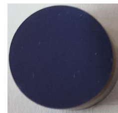
1.5 \mu\text{m} \text{TiN} deposited on CoCr by DC sputtering
