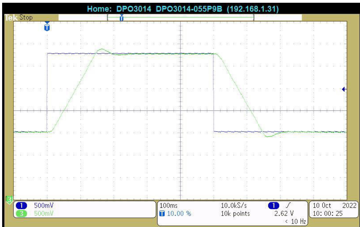
Fig. 9. Set-point and actual value of position, 70 mm step, 2-DOF PI regulator K_P=4 , T_I=100 ms, K_F=10
