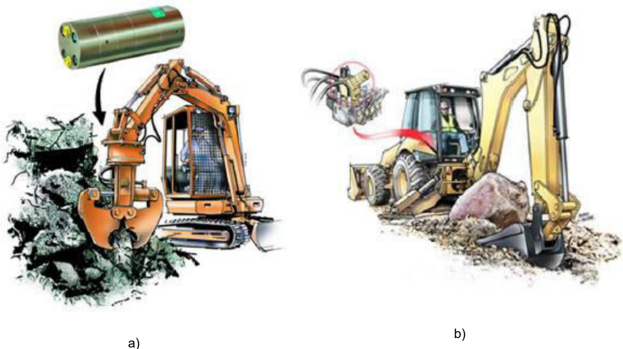
Fig. 11. Pressure intensifiers mounted on construction machinery [6]
