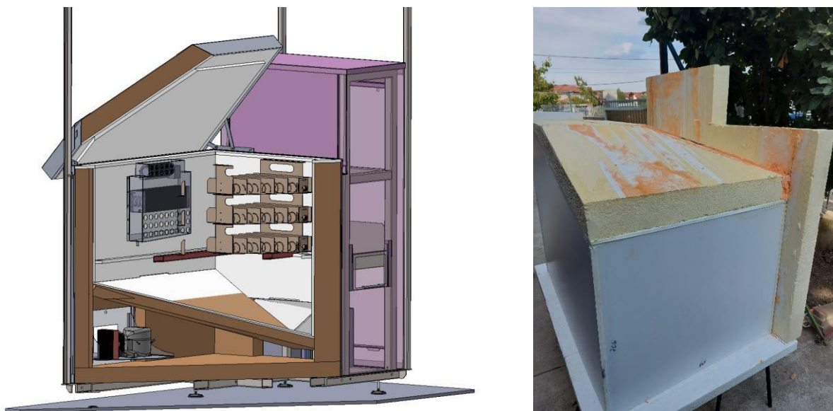
Fig. 8. Realization of a thermally insulated enclosure
