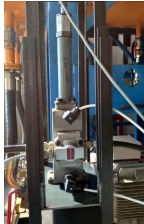
Fig. 1. Hydraulic servo cylinder equipped with transducers
