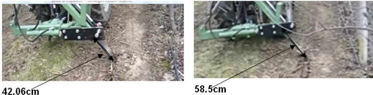
Fig. 4. The comparison on root cutting machine of cutting depths, depending on the position of the working apparatus
