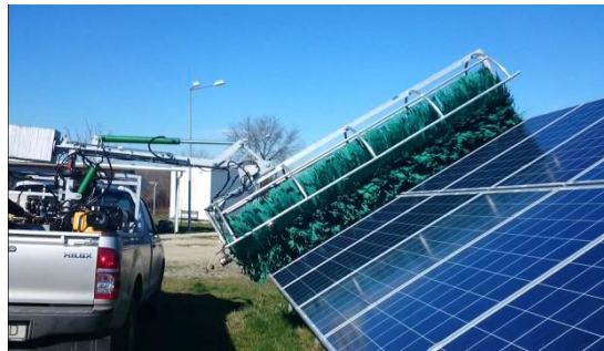
Fig. 6. Washing photovoltaic panels machine with smart distance control from the panel, made of INOE 2000-IHP [6]
