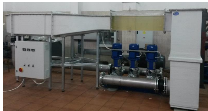
Fig. 9. Experimental stand for testing axial hydraulic turbine models
