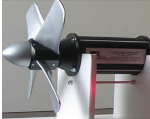
Fig. 1. Micro-hydrokinetic turbine developed in CEEX project no. X2C17/2016 [1]
