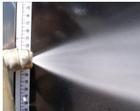
Fig. 3. Determining the angle of dispersion at the pesticide liquid to the level of nozzle
