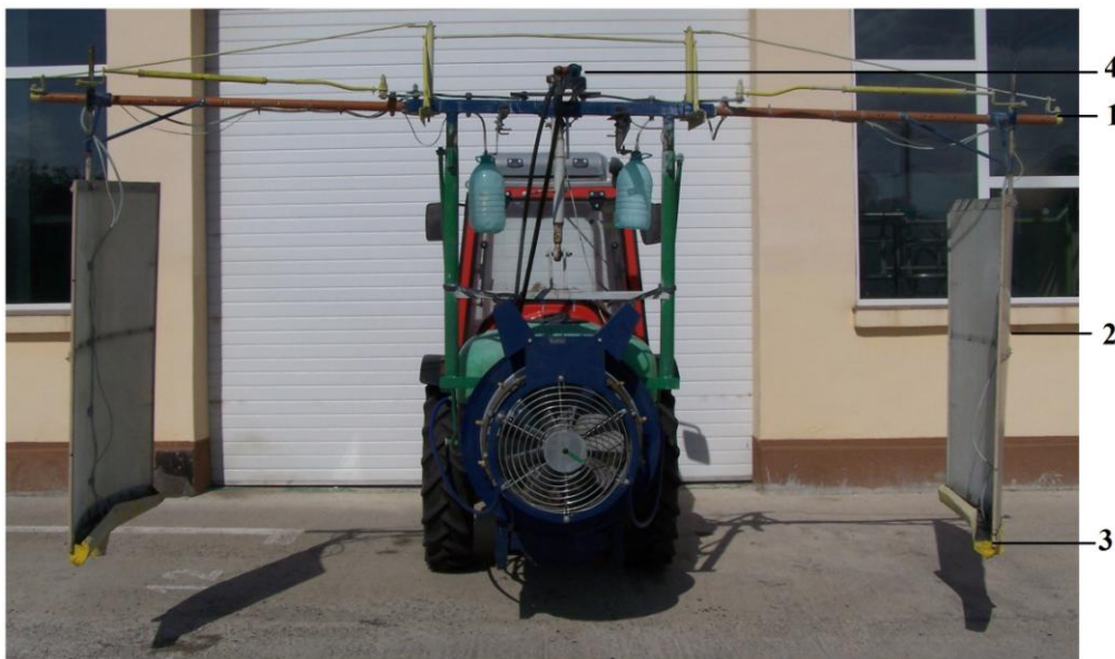
Fig. 1. Aggregate for pest and disease control with equipment to recover the dispersed liquid pesticide
