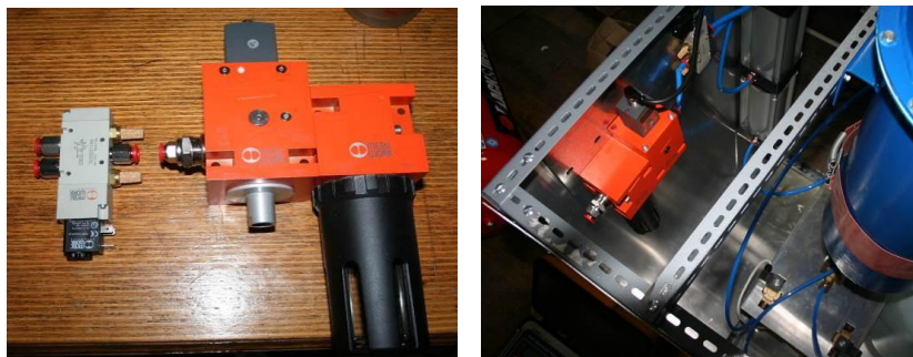
Fig. 3. Pneumatic distributor, pneumatic controller and filter Metal Work
