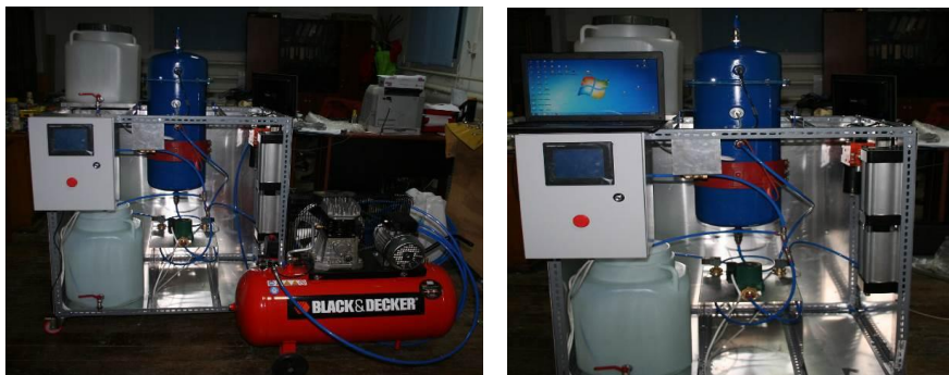
Fig. 1. Experimental model for obtaining organic fertilizers / insecticides, EXTBIO
