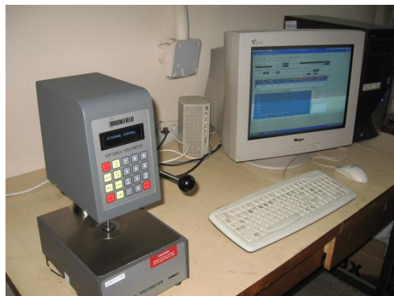
Fig. 1. Brookfield cone-plate viscometer
