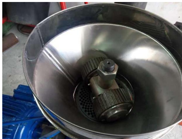
Fig. 8. Presser chamber of the pelletizing equipment
