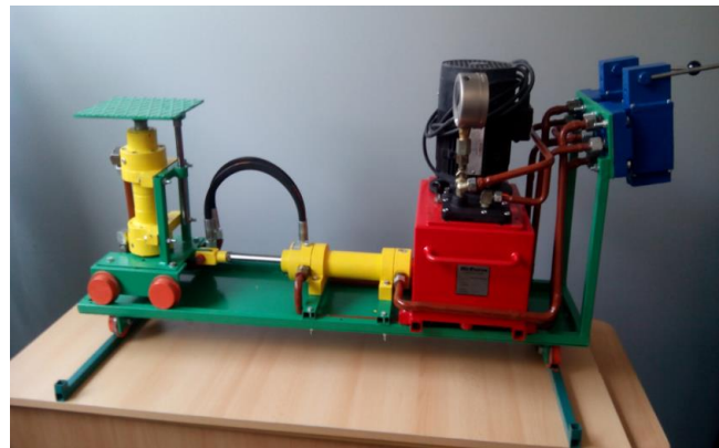
Fig. 1. Hydraulic mounting system of laminar cylinder cassette ArcelorMittal version (a); laboratory version (b)
