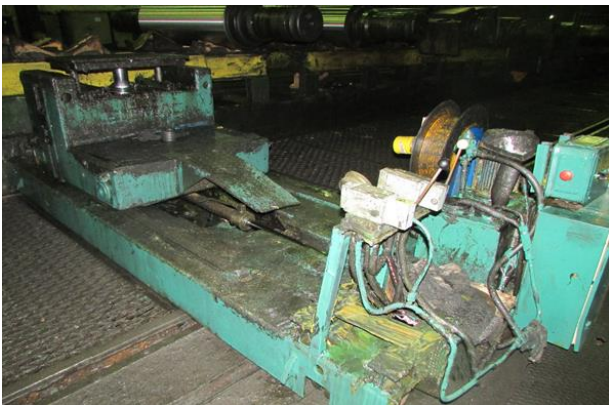
Fig. 1. Hydraulic mounting system of laminar cylinder cassette ArcelorMittal version (a); laboratory version (b)
