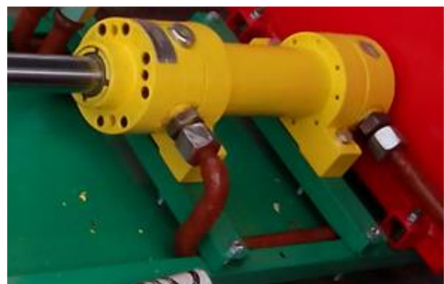
Fig. 2. Hydraulic cylinder for horizontal movement
