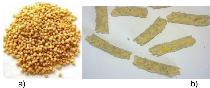
Fig. 2. Material images (soybean seeds) at the installation inlet and outlet (final product “full fat soybean”) a- Soybean seeds before processing; b- Final product “Full fat soybean”
