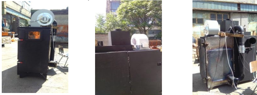
Fig. 6. The hot air generator prototype on the principle of TLU
