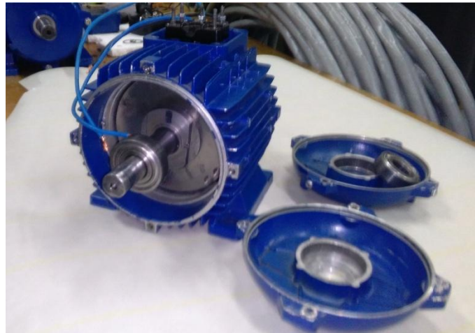
Fig. 10. Electric motor with axial air gap
