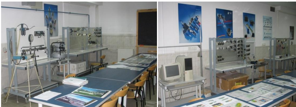
Fig. 10. Test rigs with a set of elements for pneumatic control systems
