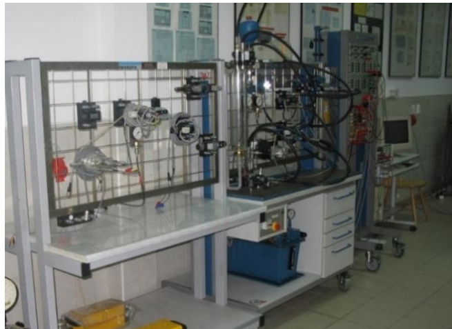
Fig. 9. Educational stand with hydraulic components and electrical and proportional control panel
