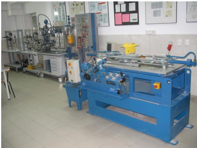
Fig. 13. Linear hydrostatic drive simulator
