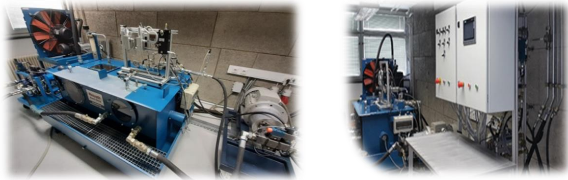
Fig. 7. Central hydraulic power unit with control cabinet
