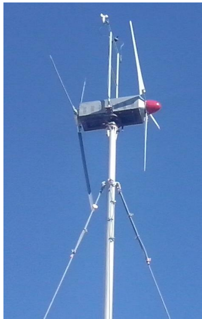
Fig. 11. Experimental model of the counter rotating wind turbine [15]
