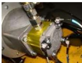
Fig. 17. Positioning of the accelerometers on the pump
