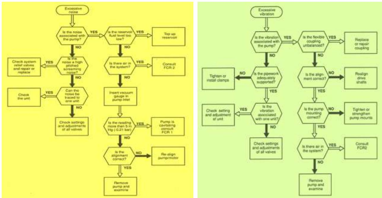
Fig. 2, Fig. 3 (from left to right) Hydrostatic pumps tested for excessive noise and for excessive vibration [7]
