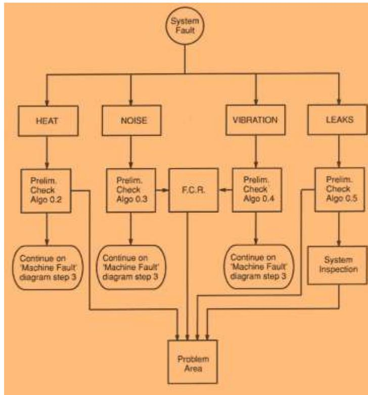
Fig. 1. Flowchart for faults that may occur in a hydraulic system, [7]
