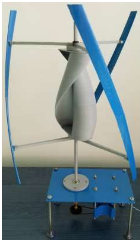
Fig. 5. The prototype of vertical axis wind turbines (1:5 scale)
