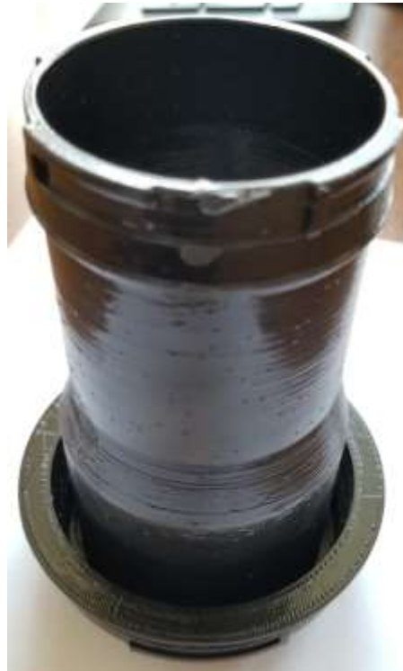
Fig. 10. Surface quality after vapor smoothing process
