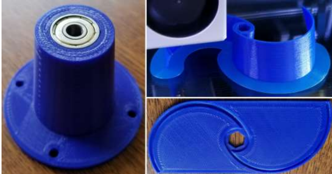
Fig. 4. Components that did not need support material during the printing process.
