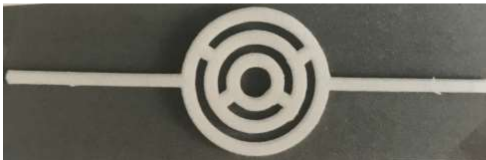
Fig. 3. Compressed air dispersion device build on the 3D printer
