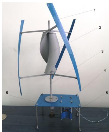
Fig. 7. The wind turbine of the demonstration model of electric combined system
