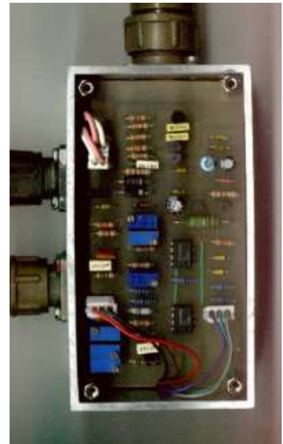
Fig. 6. Mode of manufacturing for the controller for proportional elements
