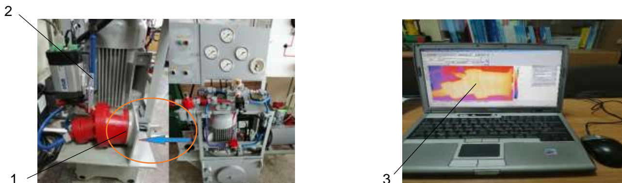
Fig. 3. Hydrostatic plant with camera thermography: axial piston hydraulic motor (1); FLIR ThermoVision A20M infrared thermal camera (2); ThermoCAM Researcher Professional specialized software for acquisition and processing of thermograms (3)
