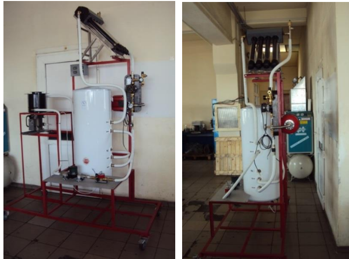
Fig. 3. The experimental model of combined thermal system
