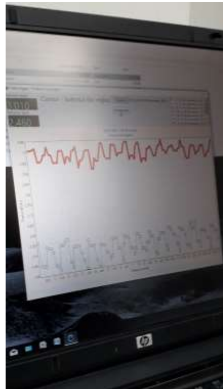
Fig. 7. Acquisition of data regarding the variation of pressures in the connection points of the device to the main pipe of the stand (the equivalent of the main pipe of the localized irrigation system)
