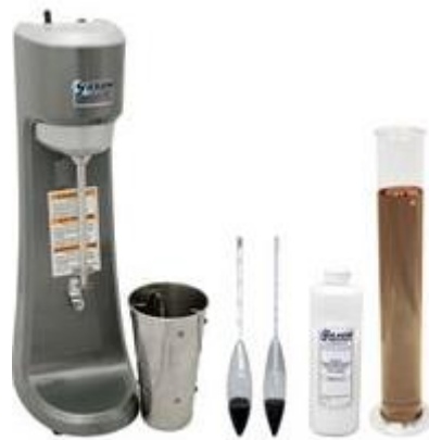
Fig. 8. Hydrometer analysis of soil
