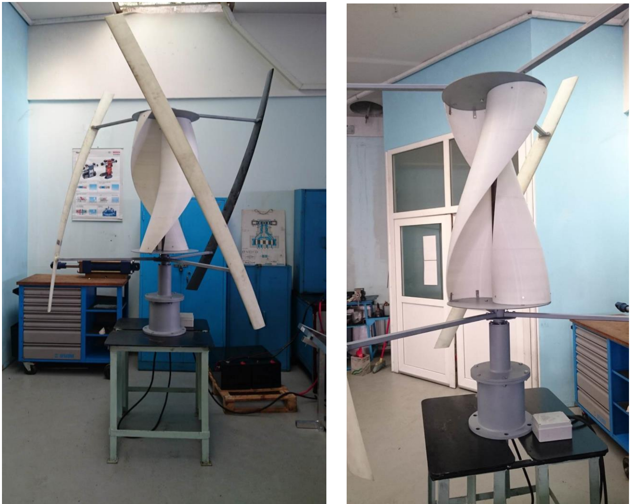
Fig. 12. Experimental prototype of the vertical-axis hybrid wind turbine
