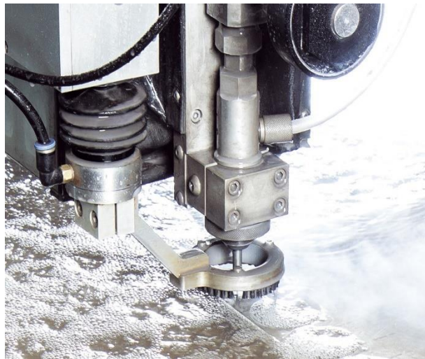
Fig. 3. CNC machining cutting with water jet
