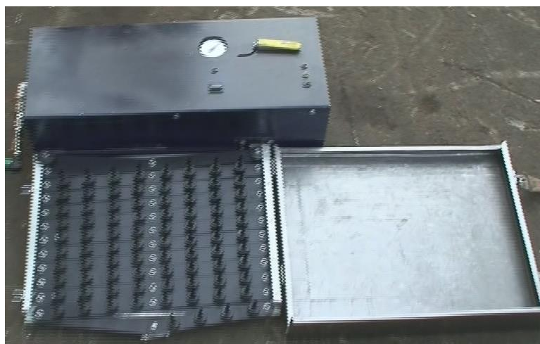
Fig. 2. Extendable, remote controlled portable barrier for stopping vehicles by controlled tire deflation
