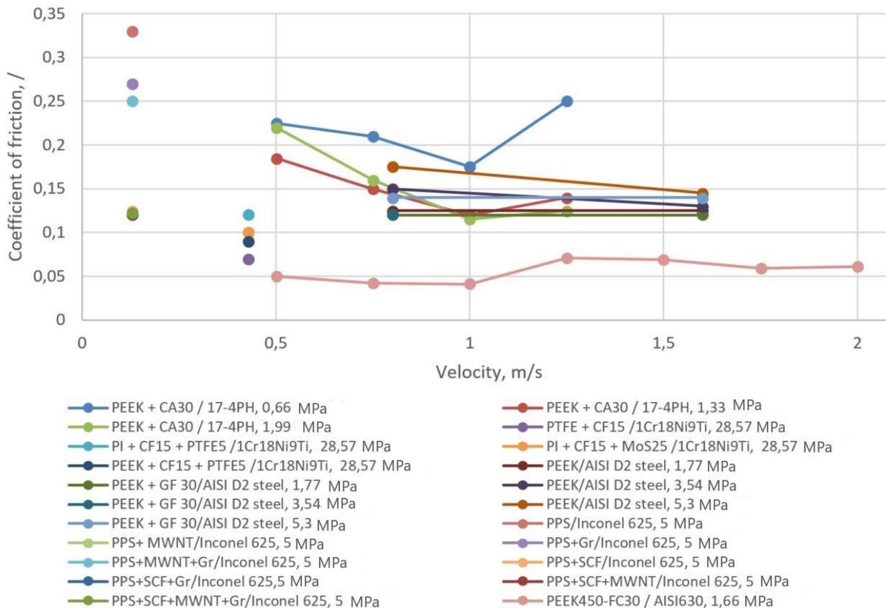
Fig. 4. An overview of tribological results for different polymers in water [17-21]
