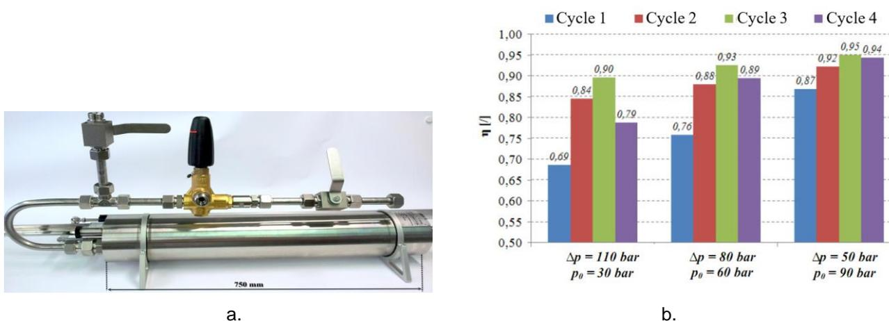
Fig. 10. a) Prototype of a piston-type water-hydraulic accumulator, b) Influences of different nitrogen pre-filling pressures for all four cycles on the water-hydraulic accumulator efficiency
