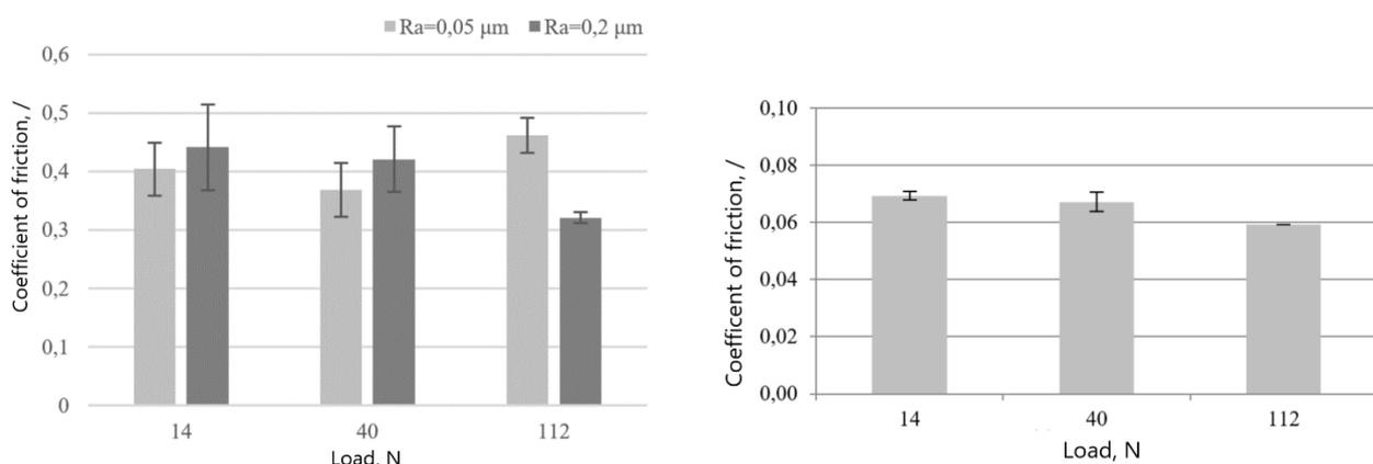
Fig. 6. Coefficient of friction in water a) AISI 440C/AISI440 , b) coating DLC / AISI 440C
