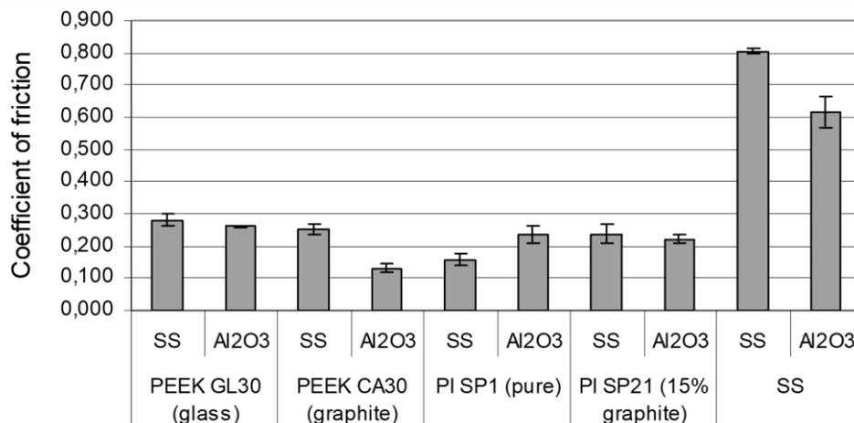
Fig. 5. Coefficient of friction for selected material pairs (SS and Al<sub>2</sub>O<sub>3</sub> pins against four different disc materials is shown)
