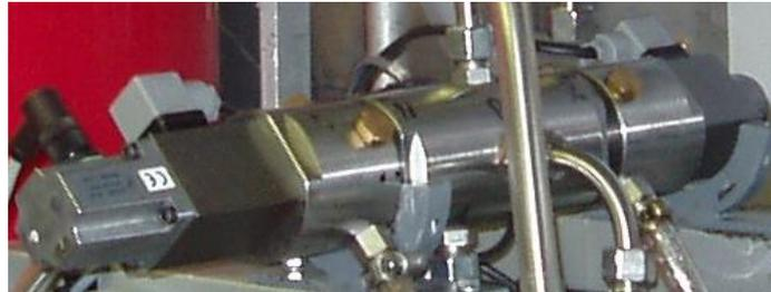
Fig. 7. Prototype of proportional directional control valve for water hydraulics
