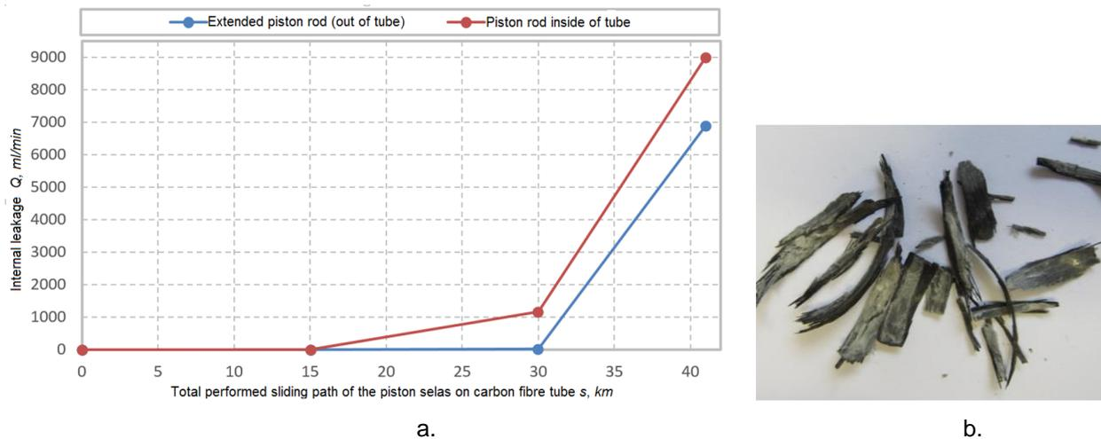
Fig. 9. Results of long-term tests of carbon-fibre hydraulic cyl. tube, a. internal leakage, b) wear
