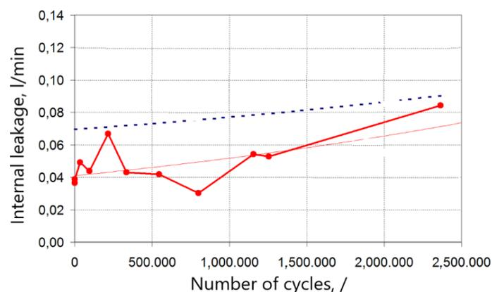
Fig. 8. Results of leakage during long-term tests of proportional water directional control valve
