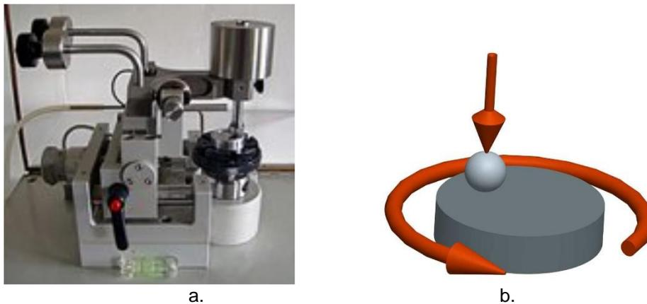
Fig. 1. a) CSEM pin-on-disc, b) testing principle
