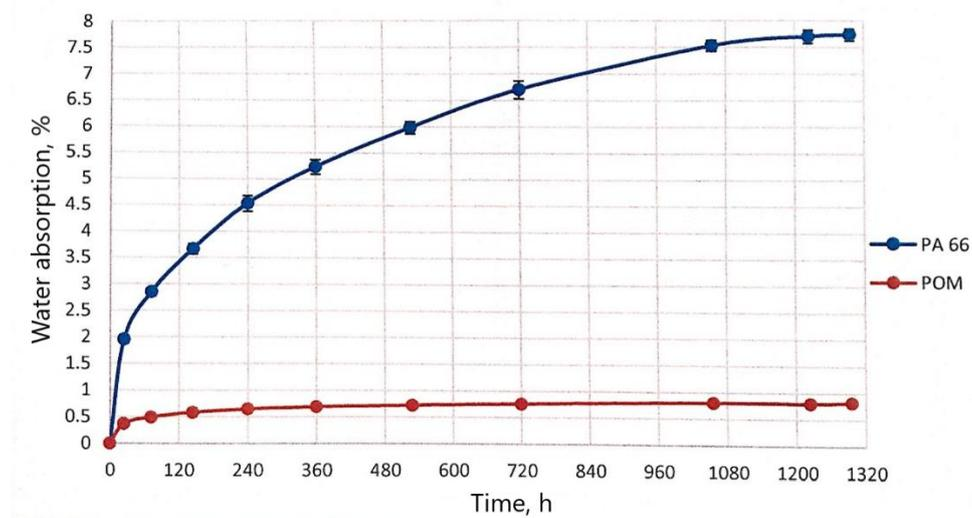
Fig. 3. Water absorption for POM and PA 66 [16]
