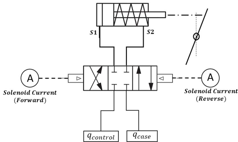
Fig. 7. Electric Proportional Pump Swash Control
