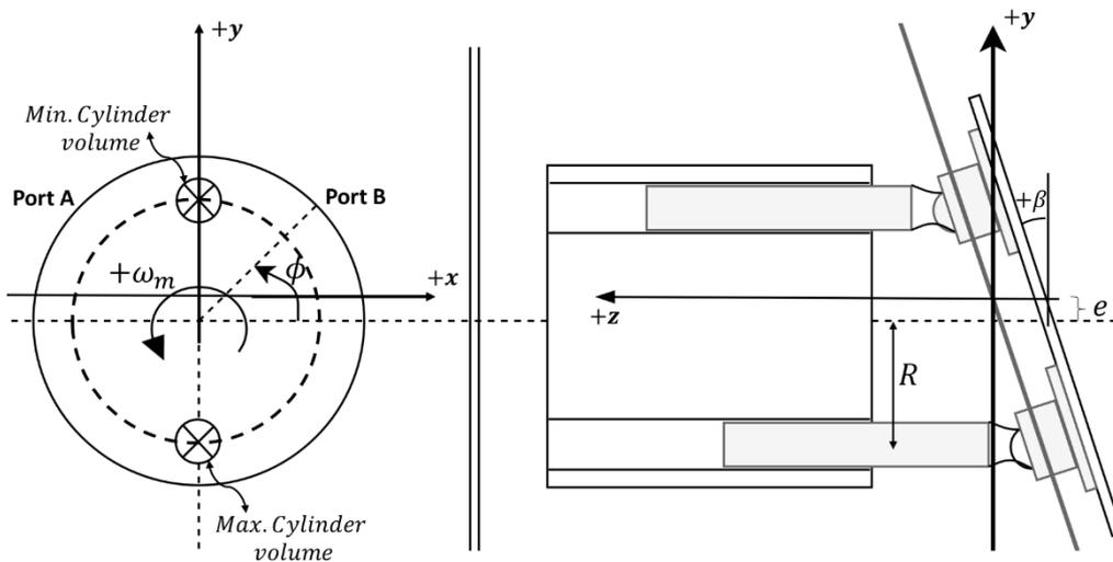
**Fig. 8.** Schematic diagram of motor RG kit with assigned sign convention
