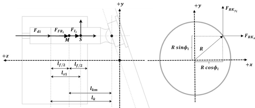
Fig. 10. Piston free body diagram for motor torque computation
