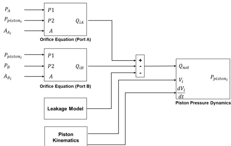
Fig. 3. Piston pressure dynamics model for pump
