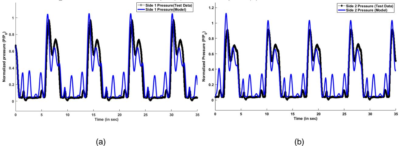
Fig. 14. CC circuit side 1 pressure (a) and side 2 pressure (b) validated with test data
