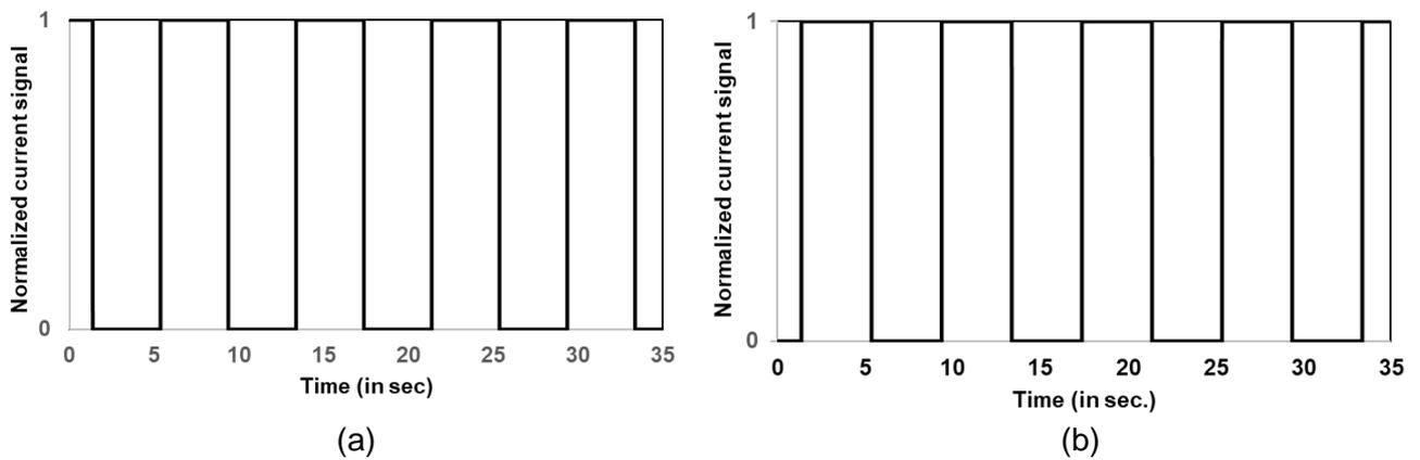
Fig. 12. Forward solenoid current signal (a) and reverse solenoid current signal (b)
