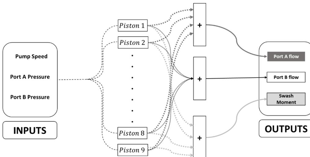
**Fig. 5.** Schematic overview of bidirectional pump mathematical model
