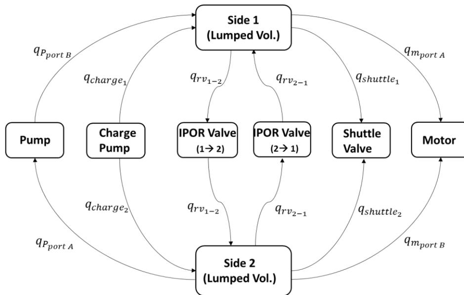
Fig. 11. Schematics of integrated CC circuit system model
