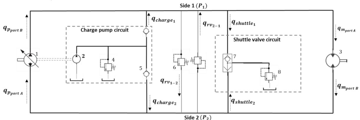
**Fig. 1.** Hydraulic schematic diagram of closed loop circuit in HST
