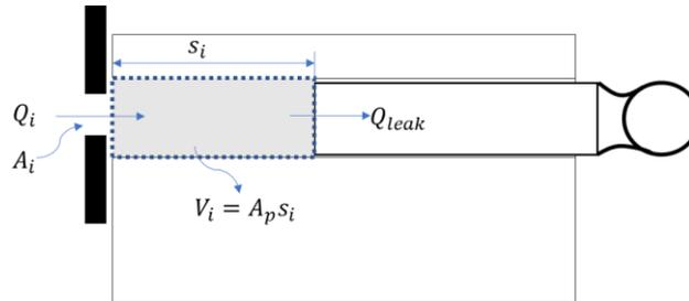
**Fig. 4.** Piston-barrel control volume
