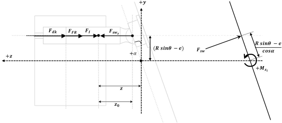
Fig. 6. Piston free body diagram for pump swash moment
