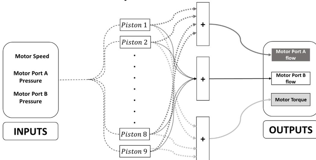
Fig. 9. Schematic overview of bidirectional motor model
