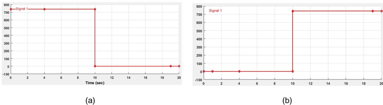
Fig. 15. Forward (a) and reverse (b) solenoid current
