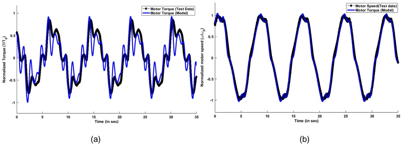
Fig. 13. Normalized motor torque (a) and motor speed (b) validated with test data
