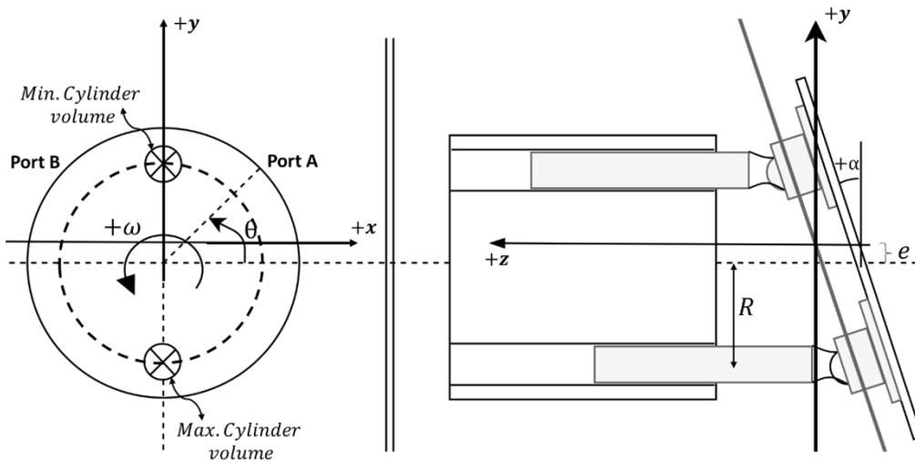
Fig. 2. Schematic diagram of pump RG kit with assigned sign convention
