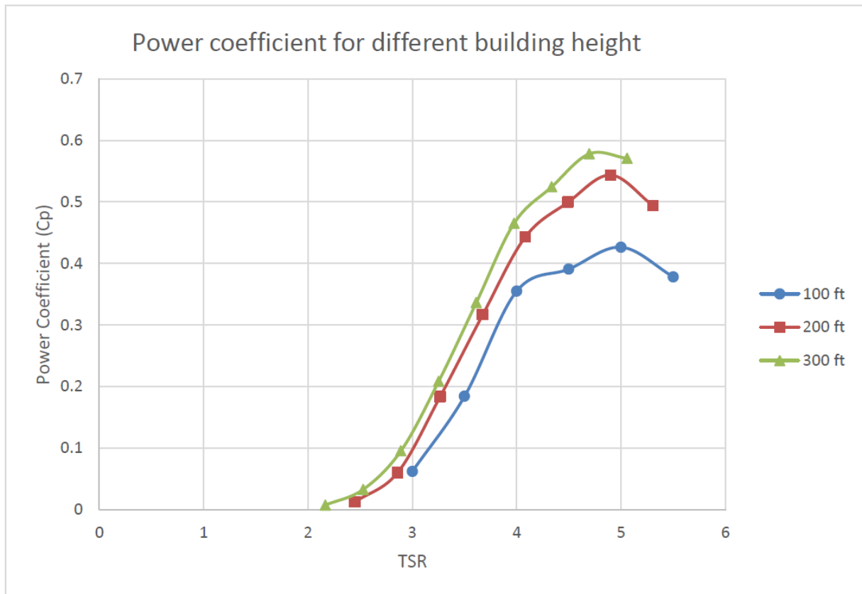
Fig. 10. Power coefficient ( C_p ) for different building heights to varying values of TSR
