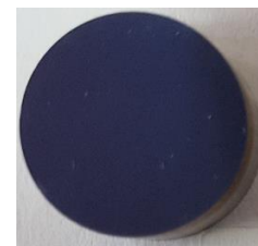
1.5 \mu\text{m} TiN deposited on CoCr by DC sputtering
