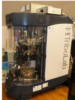
Fig. 2. Ball on disc tribometer
