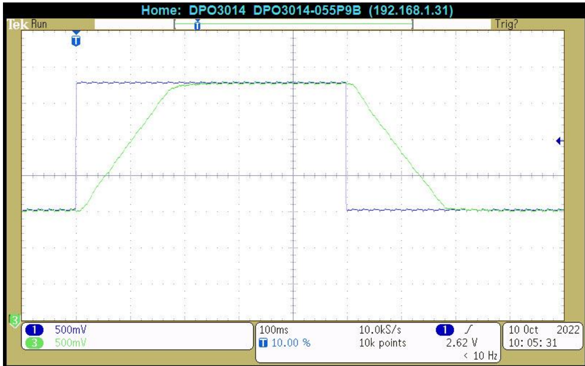
Fig. 8. Set-point and actual value of position, 70 mm step, 1-DOF PID regulator K_P=4 , T_I=100 ms, T_D=10 ms
