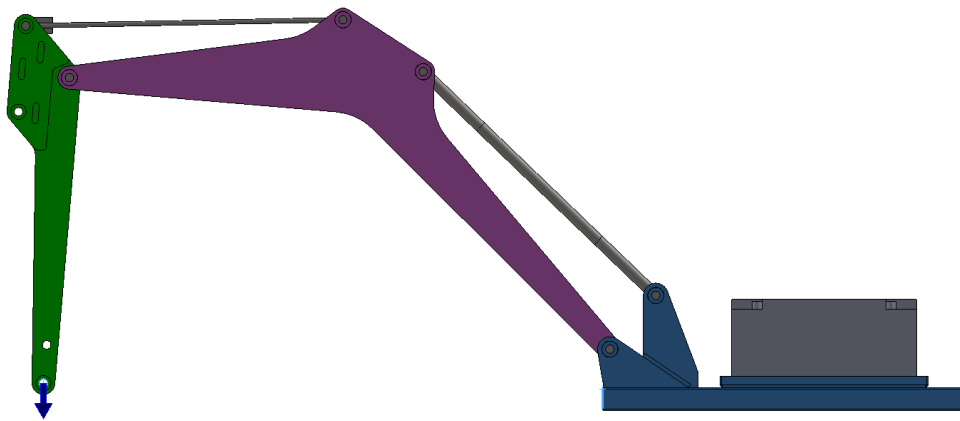
Fig. 19. 1000 N load applied to the final joint of the excavator arm
