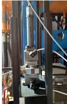
Fig. 1. Hydraulic servo cylinder equipped with transducers
