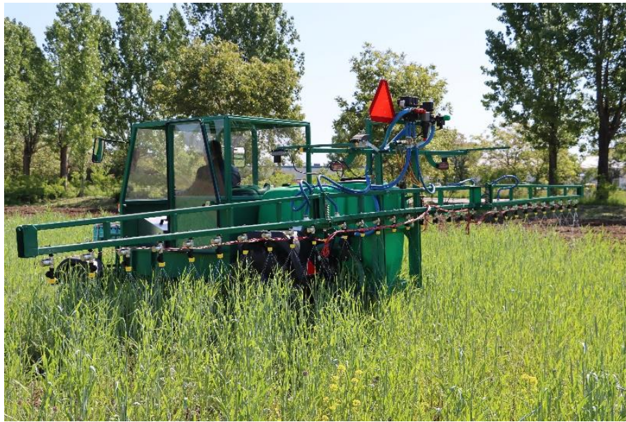
Fig. 3. Innovative system - field experiments with fertilization nozzles
