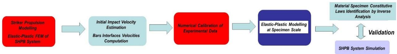
Fig. 9. Flowchart of proposed hybrid analytical-numerical analysis of SHPB system using numerical calibration, entire SHPB Finite Element Modeling and Inverse Analysis
