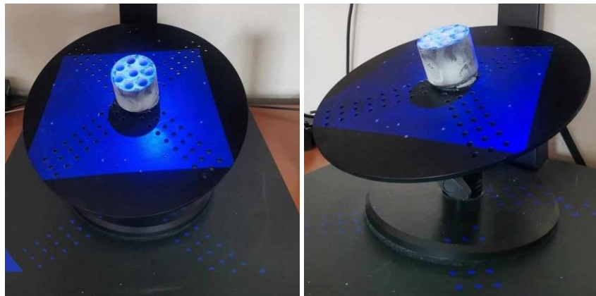
Fig. 2. Applying the anti-reflective spray and starting the scanning process of the piston block
