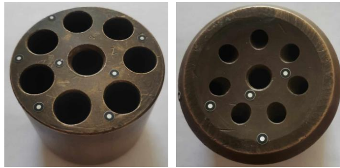
Fig. 1. Applying reference markers to the piston block
