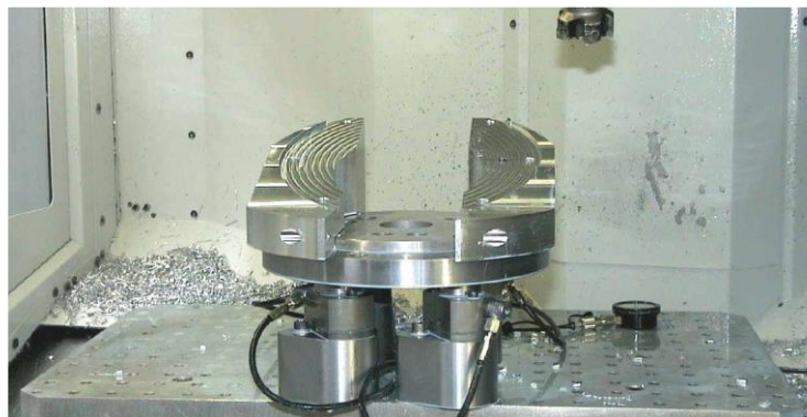
Fig. 2. Clamping a complex blank on a 5-axis CNC machining center
