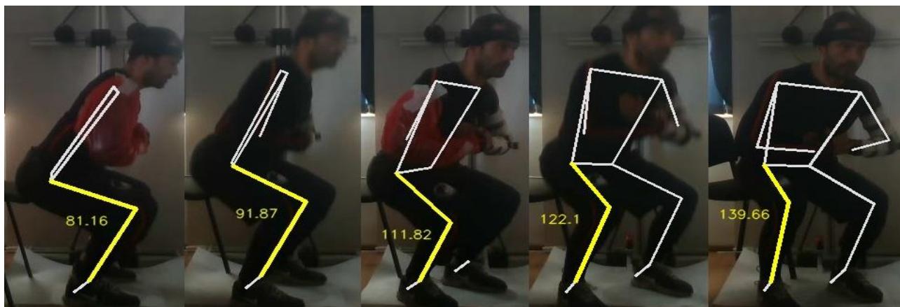
Fig. 2. Successive positions of the human subject for measuring the right knee joint flexion angle
