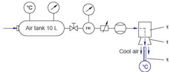
**Fig. 3b.** Compressed air cooling circuit by expansion in a centrifugal field
