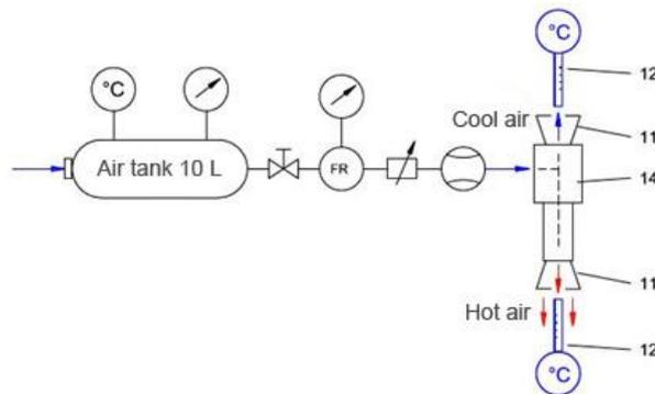
**Fig. 3c.** Compressed air cooling and heating circuit with vortex tube / Ranque-Hilsch
