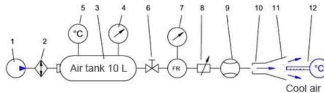
**Fig. 3a.** Compressed air cooling circuit by free flow from the tube
