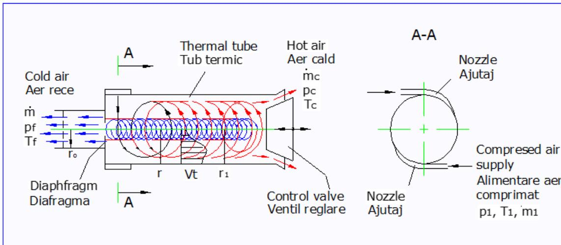
**Fig. 2.** Gas-dynamic phenomena in the Ranque-Hilsch tube
