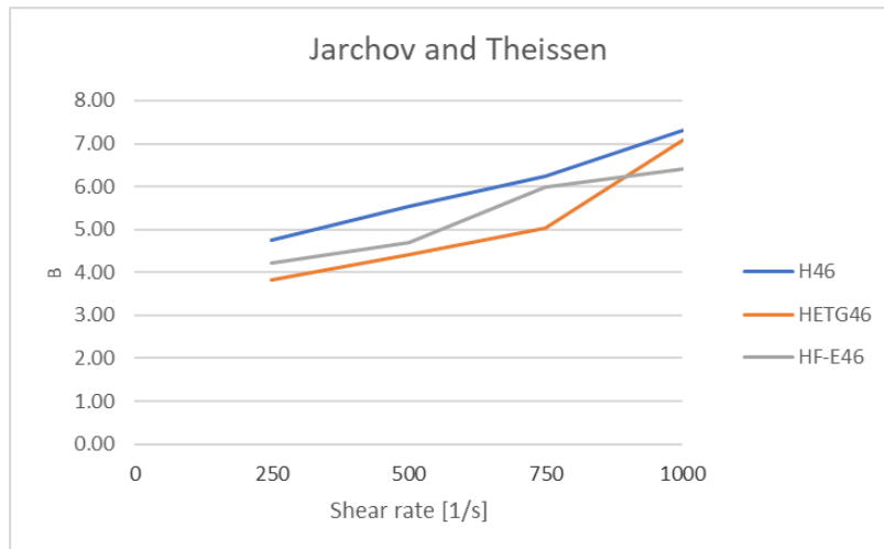
Fig. 11. Variation of the rheological parameter of the Jarchov and Theissen thermal model depending on the shear rate for the three hydraulic oils
