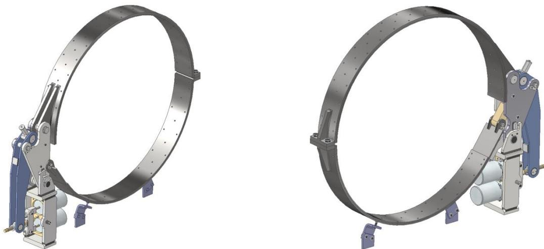
**Fig. 10.** Graphical modeling of the pneumatic braking system for industrial winches
