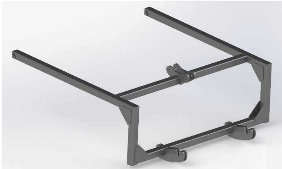
Fig. 2. The three-dimensional geometric model of the subassembly "Seeder support" - isometric view
