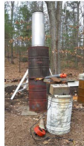
Fig. 8. Artisanal biochar and heat production system made by Jolly Roger
