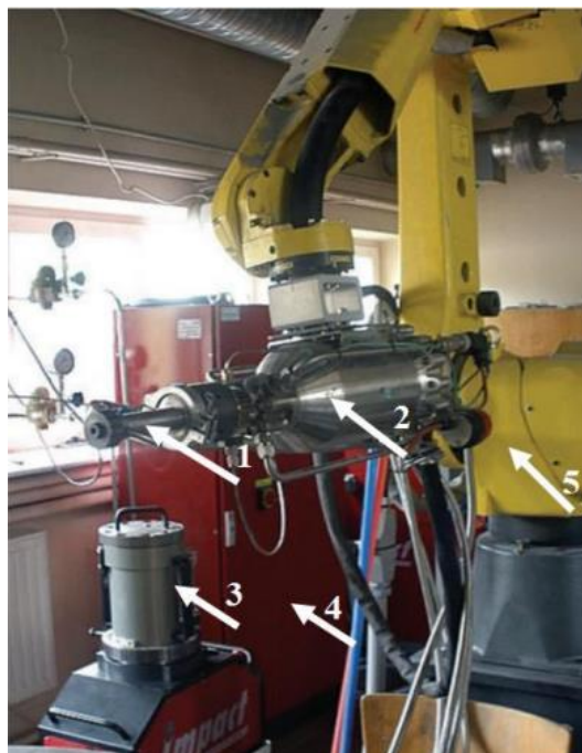
Fig. 4. The Cold Gas spraying coating system setup [7]
