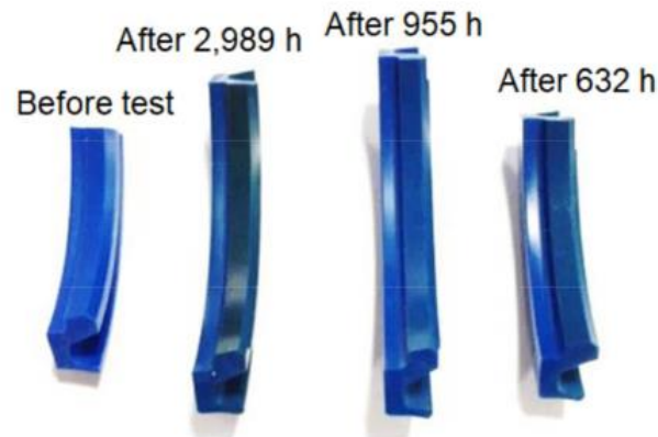
Fig. 2. O-rings before testing, after 2989, 955 and 632 hours [15]
