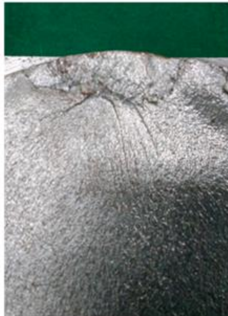
Fig. 1. Cracked surface of the piston rod, followed by component failure [14]
