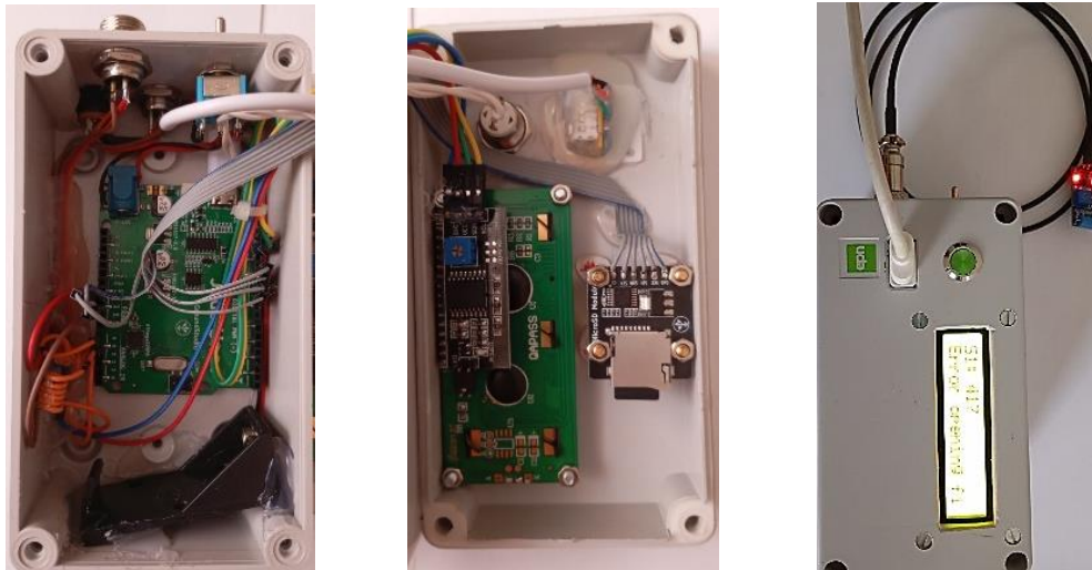
Fig. 6. Experimental setup of low-cost gear pump vibration monitoring system
