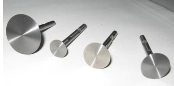
Fig. 5. Geometry of Brookfield viscometer
